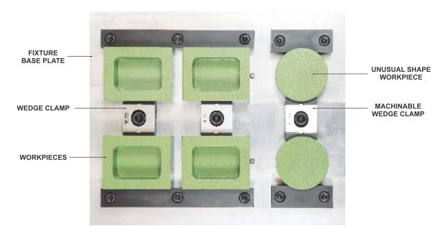
If your workpiece is suitable for clamping with 'TOOLFAST' Wedge clamps, our team can design and manufacture a multiple clamping fixture for you as the one shown in the picture.
