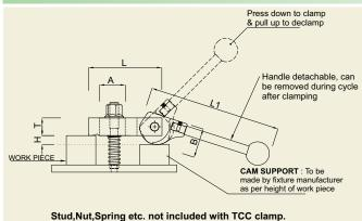
Most ideal for quick Hold Down Clamping in fixtures. Conventional Strap Clamps in fixtures can be replaced by these quick acting Cam clamps without much effort. These clamps have high clamping force suitable for machining fixtures.
